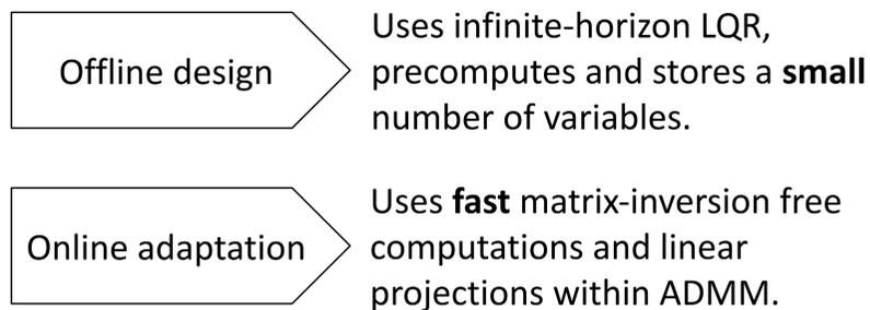
TinyMPC shows a **higher speed and smaller memory footprint**, compared with the state-of-the-art OSQP [2] on **microcontrollers**.
